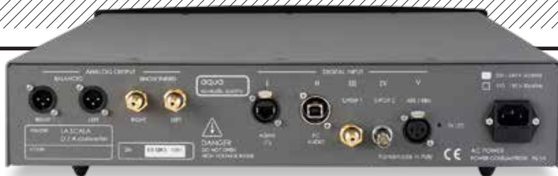
ABOVE: The La Scala MkIII's digital inputs are S/PDIF (RCA and BNC), AES/EBU (XLR), USB-B for computer connection and IP's 'AQLink' (RJ45). Fixed analogue outputs are offered on single-ended (RCA) and balanced (transformer-coupled XLR) connections
